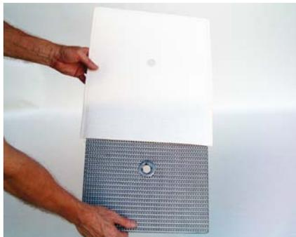
3. Attach suction pipe and plate with top and bottom plate coupling. Make sure coupling is completely fastened. You should not be able to turn the envelope when coupling is secure.
