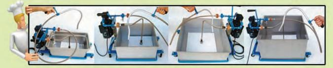
Motor 1/3 H.P. 60 cycle 110-V 5 amp 1 phase temperature 400° F heavy duty.
